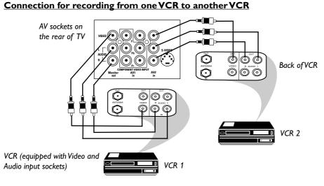
Connect the sockets of the VCR which you wish to record from, to the corresponding sockets at either AV1 or AV2
